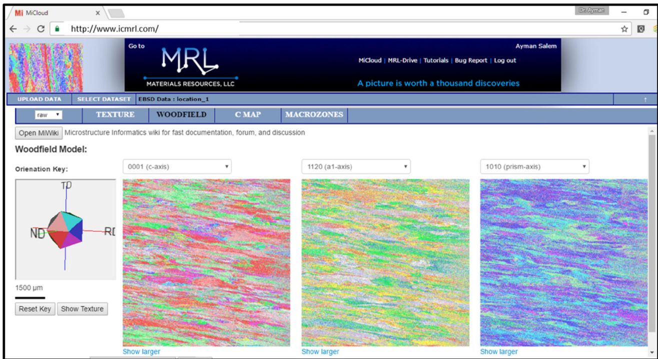
Fig. 12 EBSD data colored according to Yamrom's method [48] to reveal MTR using Woodfield app on MiCloud (Color figure online)
